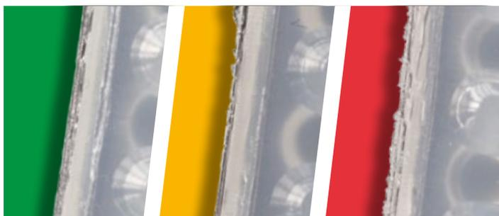
■ Clamping force Bekum optimized ■ Clamping force speeds up ■ Clamping force standard
