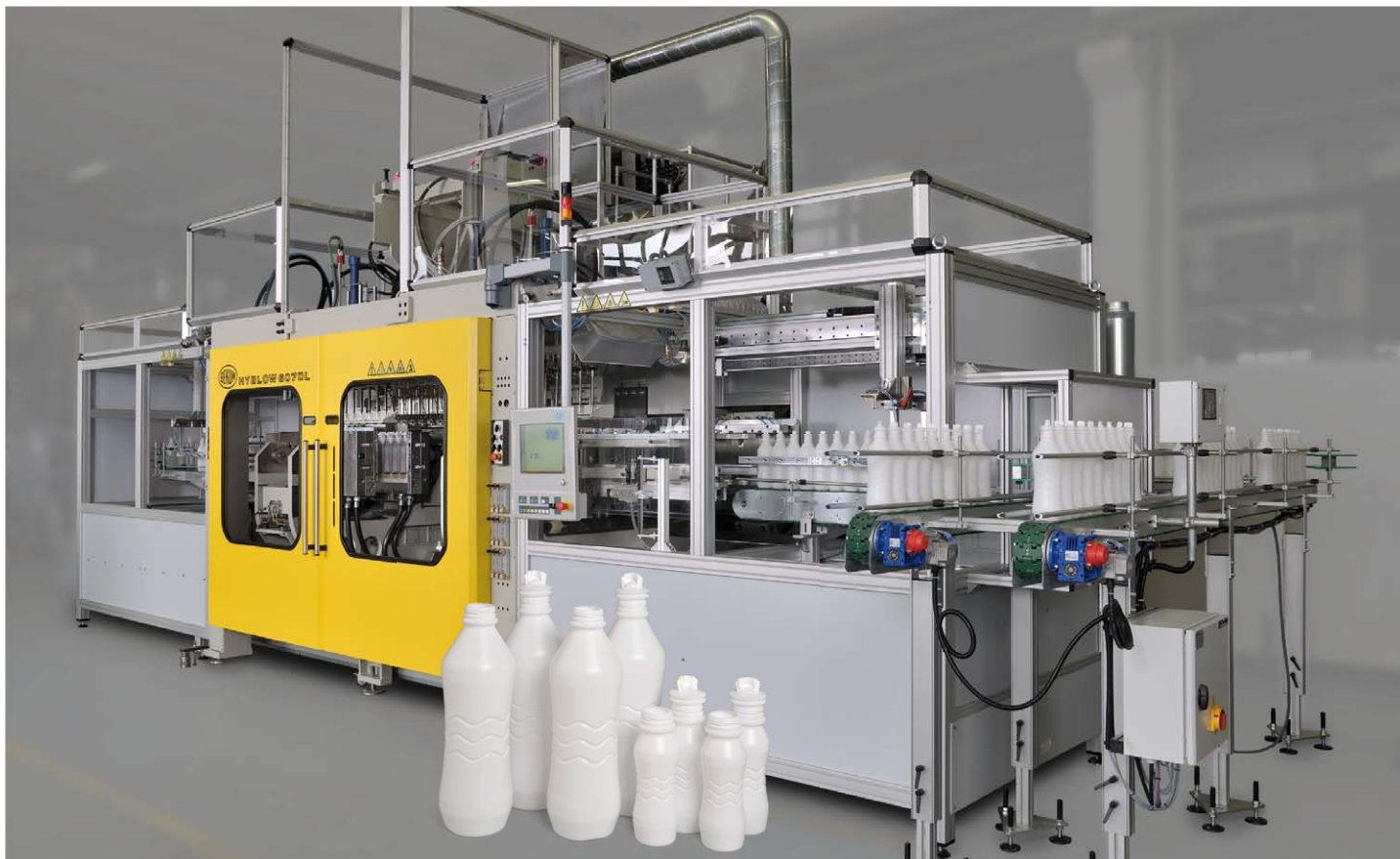
HYBLOW 607 DL for the 9-fold production of 1000 ml milk containers with production samples
